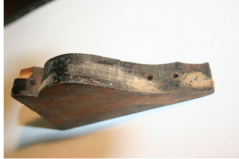
Showing saw marks on the curved surfaces
