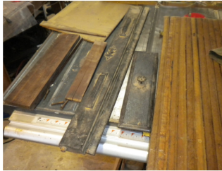
Tambour door slats, middle piece with handles is lock slat, on right are 1 inch wide slats shown from back side
