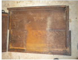
Desk top with glue joint separated
