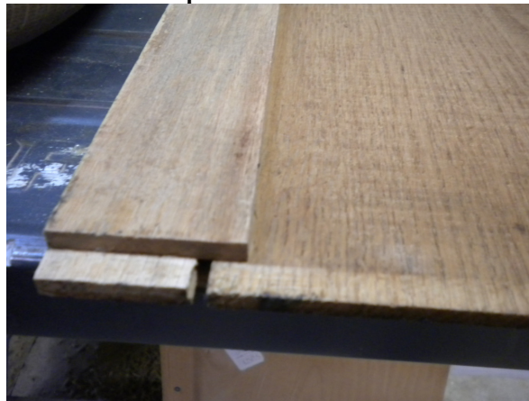
Back panel showing vertical saw marks
