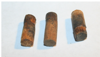
These 7/16 inch dowels were used to locate the tambour door assembly
