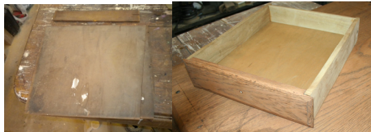
Damaged drawer bottom and back, drawer with new parts added
