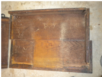
Desk top showing separated joint
