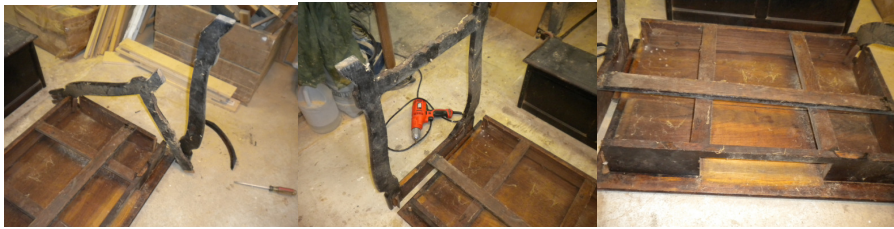
Desk top assembly showing legs coming apart
