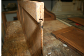
This is back panel 1/4 inch thick solid oak
