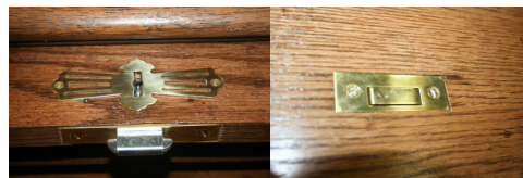
New lock installed on Tambour lock slat, and strike plate on desk top
