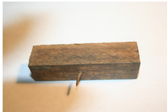
Corner brace with nail protruding
